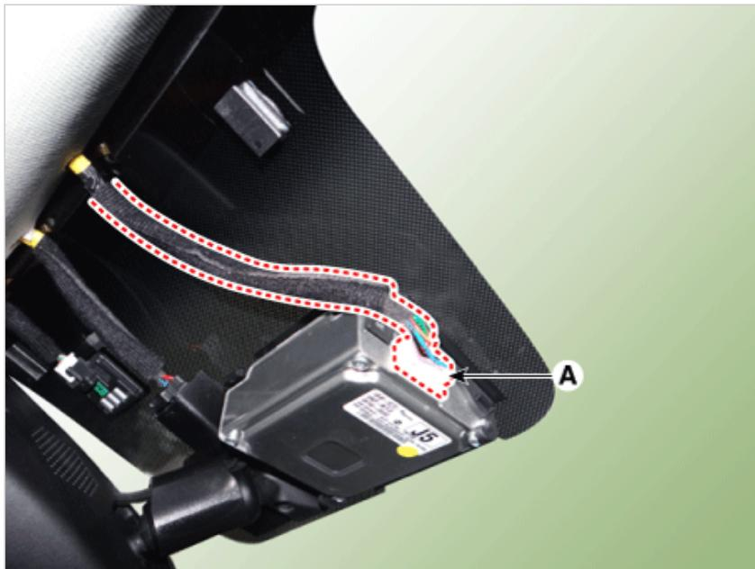
4. Remove the LKA unit (B) by pulling out lock pins (A).
